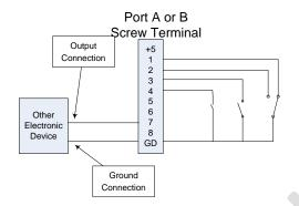
Switches, relay contacts, etc are simply wired between Ground and the relevant input screw terminal. There is a Ground screw terminals on the end of each of the Port A and Port B screw terminals marked GD shown on the right above.
