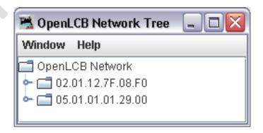
Each node has a unique address assigned at manufacture time. The LCP1 node address is the serial number printed on the board near the top. In this example we will configure the node with address 05.01.01.01.29.00. Open the node and it will reveal various information and a folder of supported protocols.
