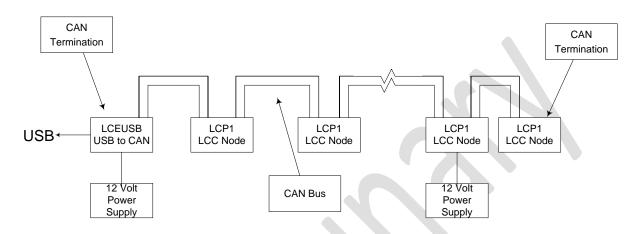
The diagram above shows several nodes connected by a daisy chain CAN segment. The power supplies can be connected in any convenient location. For small current loads, only one supply may be necessary.
